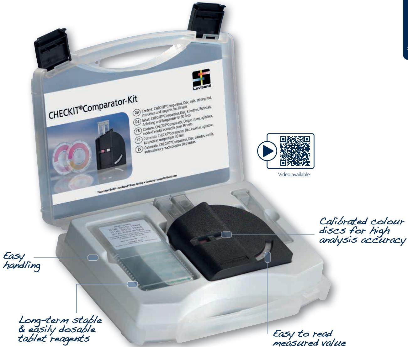
CHECKIT® Comparator Test Kits are accurate, easy to use test kits for water analysis. Simply add the reagent to the sample cell, rotate the disc until the colour matches the prepared water sample and read the concentration value.
