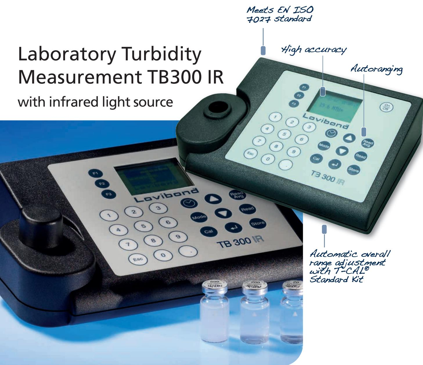
Turbidity is measured according to EN ISO 7027 by nephelometric means (90° scattered light). The infrared light-source permits measurement of coloured and colour-free samples.
