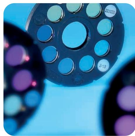
Test disc with colour-stable glass standards
